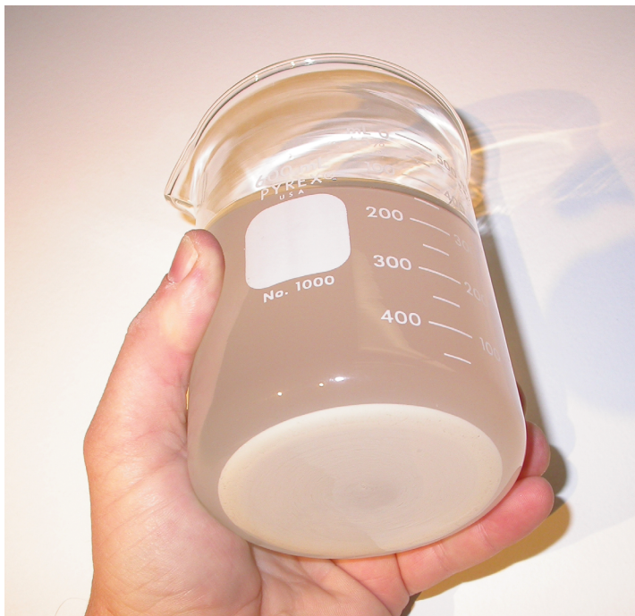
Figure 14. Several liquid spray formulations (wettable powders, suspension concentrates, and micocapsules) form true suspensions, and will settle out of water when given sufficient time. In these photographs, a suspension concentrate was diluted in water at 4 p.m. (top photograph). The following morning, the solid, particulate matter had settled to the bottom of the glass beaker (bottom photograph), and required agitation to re-suspend the product.
